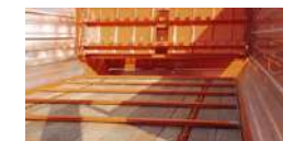
Full width floor slats ensure each load is fully cleaned out to minimise wastage. The slats are mounted to hi-tensile calibrated link chain which has been proven for years in the gritty acidic silage environment, without rusting and seizing like roller chains do.
