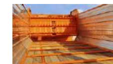
The durable hardwood floor and stainless steel sides protect against the corrosive effects of silage.
